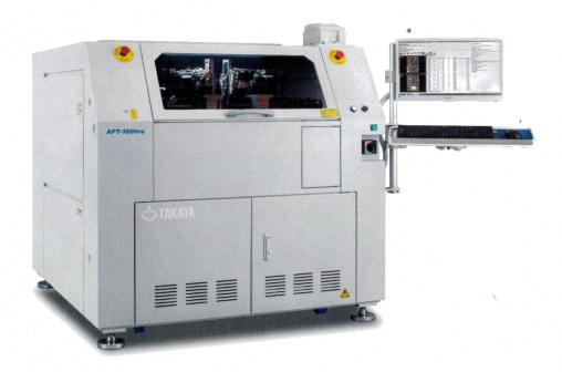
The APT-1600FD Series is a dual-sided flying probe test system that deploys the flying probes to both sides of a UUT. Owing to the dual-sided probing contact, the APT-1600FD Series can contribute to a marked increase in test coverage and also assures the shortest amount of test time.
